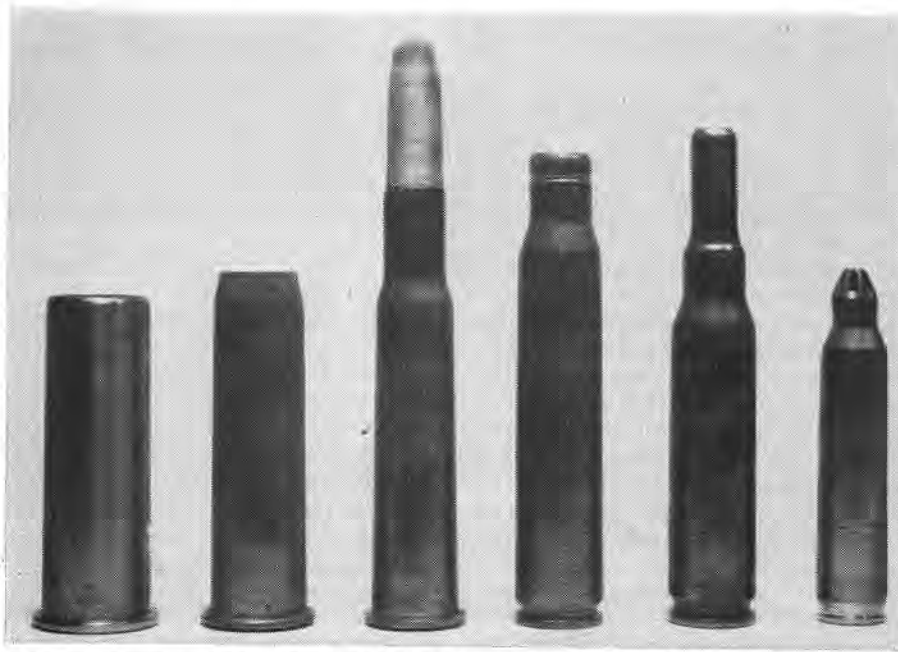
U.S. Army blank cartridges (l.-r.): .50-70 Gov't, .45-70 Gov't, .30-40 Krag Model 1896 (paper bullet), .30-'06 Model 1909, 7.62 mm. NATO M82, 5.56 mm. XM200.
