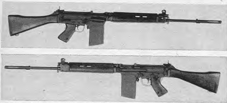
The T48, final form of the contending rifle submitted by Fabrique Nationale of Belgium and adopted by several nations. It weighs 9.7 lbs. unloaded, slightly more than the M1 rifle. Barrel length is 21". Caliber, magazine capacity, provision for semi-automatic and full-automatic fire, and flash hider are like those of M14 rifle. Gas cylinder is on top of barrel. Unusual feature is hinged action like double-barrel shotgun, permitting ready removal of action parts. Rear sight is quickly adjustable in elevation; in windage only a zeroing adjustment is provided. A heavy-barrel model with bipod was also tested
