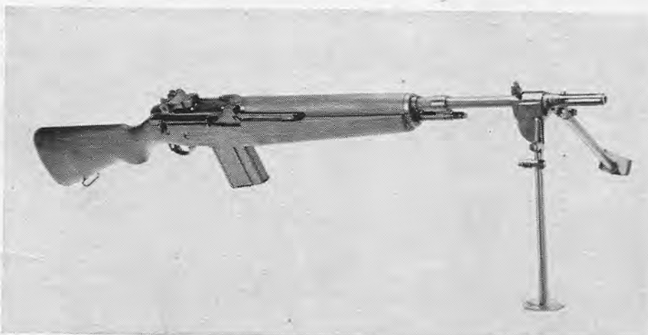
Heavy-barrel form is the Automatic Rifle M15. Its special features are a heavy barrel, muzzle bipod, butt hook, and heavier stock. The M15 will always be fitted with the change lever permitting full-automatic fire. Its weight is 14.1 lbs., or 6.7 lbs. less than the Browning automatic rifle (BAR) which it replaces
