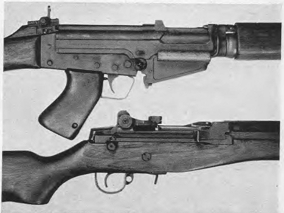
Close-up of T48 (top) and M14 rifle actions. Length of T48 receiver makes necessary a pistol grip under the action, to keep overall length of rifle within desirable limits
