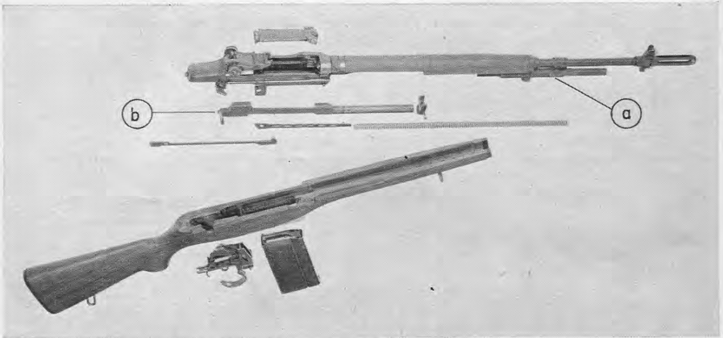
The M14 rifle is field stripped without tools. Action parts resemble those of the M1 rifle, but are markedly fewer and simpler in design. Gas cylinder mechanism (a) is of the expansion type, giving a longer and smoother push than the simple blow of the usual gas piston. Operating rod (b) is short, and gas cylinder remains attached to barrel when the rifle is dismantled
