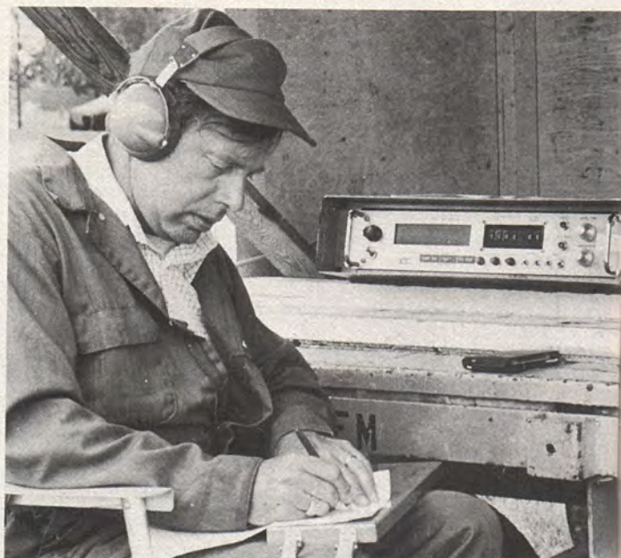
Examination of the new National Match ammunition began in 1981 at Camp Perry, where personnel and equipment from Rock Island Arsenal aided in recording the velocities of 25-shot samples.
