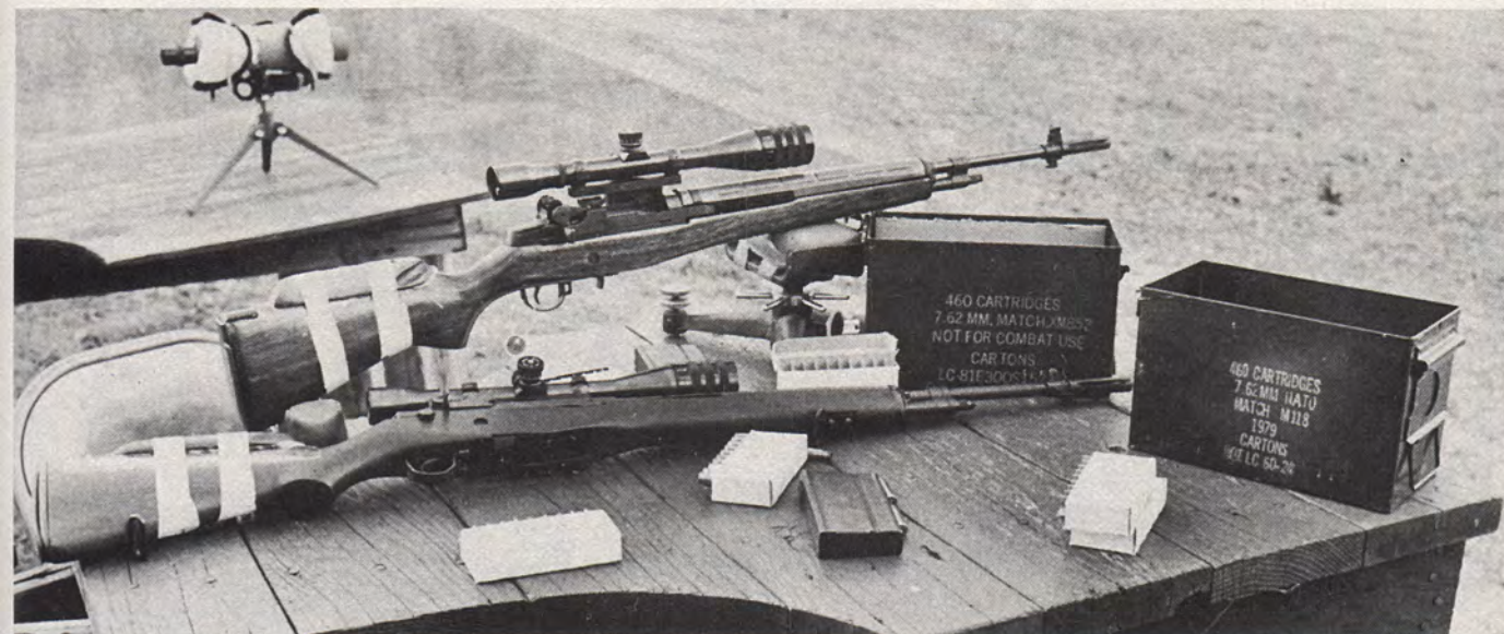
To aid in our test, the Director of Civilian Marksmanship provided a National Match M14 and sufficient M118 and XM852 ammunition for a thorough wringing out. The M14 and an accurized M1A were fitted with scopes and mounts lent by Weaver and S&K. Accuracy tests were conducted by two shooters who shared in firing five 10-shot groups with each ammunition type from each of the test rifles.
