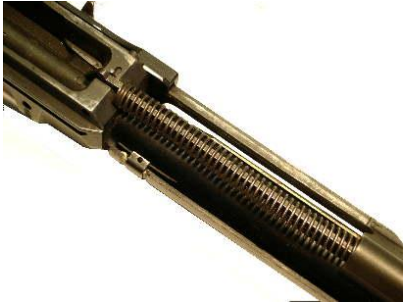
Fig. 8 Sadlak NM Spring Guide Installed
