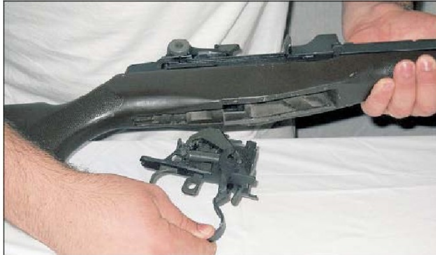
Removal of the trigger group.
